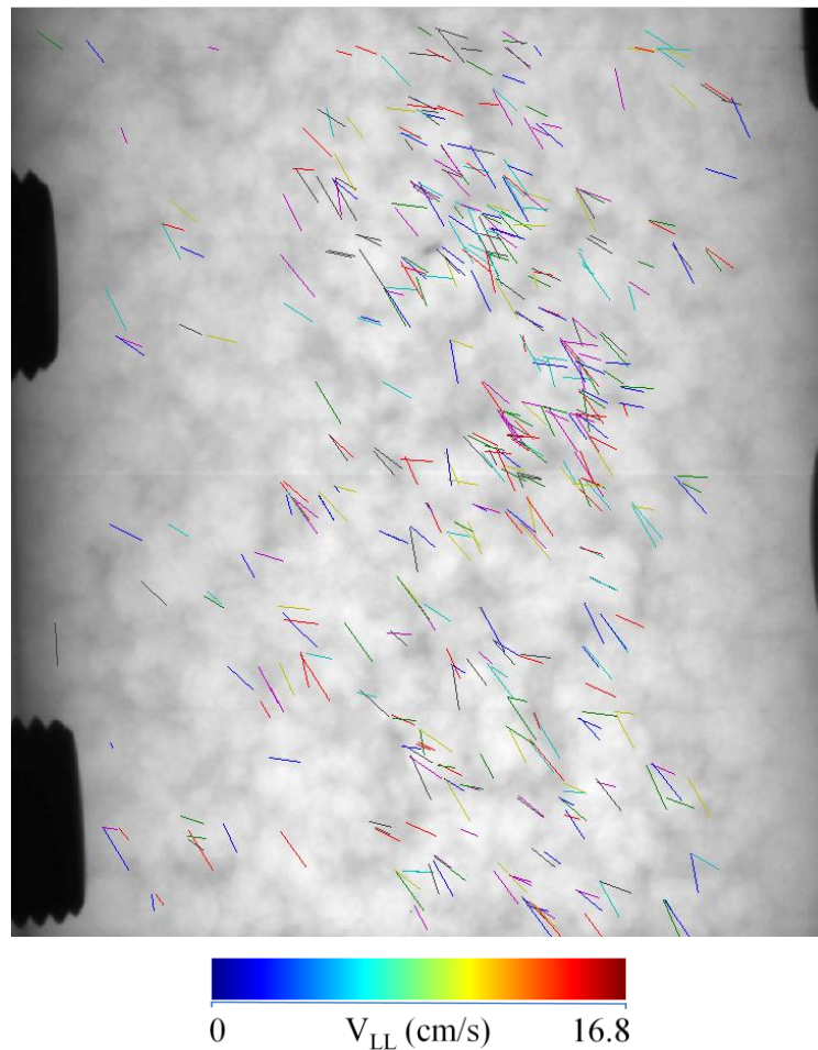
Figure 4.7. Flow patterns that were successfully tracked with the combined technique. The color bar indicates the range of obtained V_{LL}
